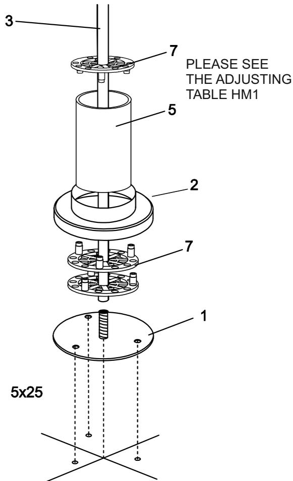
FIXING FITTINGS ON THE GROUND ARE NOT SUPPLY, THEY MUST BE CHOOSE IN FUNCTION OF FLOOR.(PLEASE TAKE PRECAUTION MEASURES IN CASE OF HEATING FLOOR).
